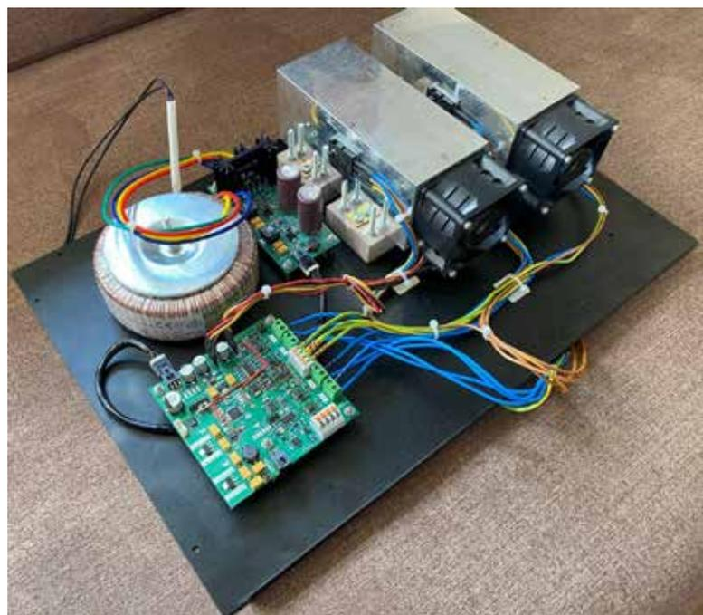
Figure 2: Prototype of the DC electronic load
